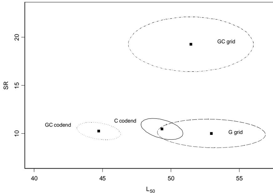
Fig. 3. The 95% confidence regions of the selection parameters for cod,  $L_{50}$  (the length in centimetres for which the estimated retention probability of the gear is 50%) and SR (selection range =  $L_{75} - L_{25}$ ), for the grid and codend (mesh) in the different experimental setups. Overlap in these confidence regions shows that selection is not significantly different between gears (gear compartments).
